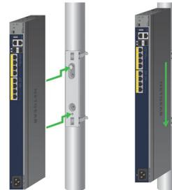
Attaching the Switch to a Rectangular Pole
