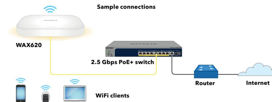
The access point receives an IP address from a DHCP server (or a router that functions as a DHCP server) in your network. If your network does not include a DHCP server, the access point uses its default IP address 192.168.0.100.
