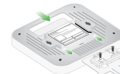
3. Slide the access point into the bracket until it locks in place. The locking tab must be at the front of the access point.
