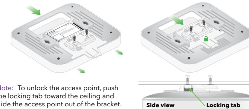
**Note:** To unlock the access point, push the locking tab toward the ceiling and slide the access point out of the bracket.
