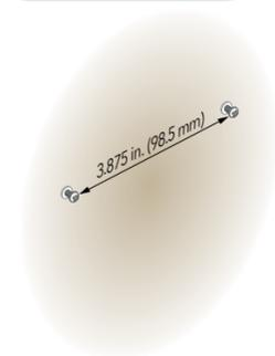
2. Line up the holes on the bottom of the access point with the screws in the wall and mount the access point to the wall.
