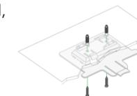
2. Hold the access point upside down with the front of the access point facing the bracket. Then, line up the guides on the bottom of the access point with the bracket.
