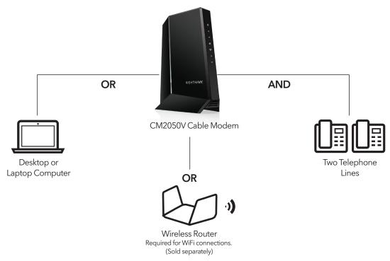
Connect the CM2050V Cable Modem directly to your computer or your WiFi router for connecting to wireless devices.
