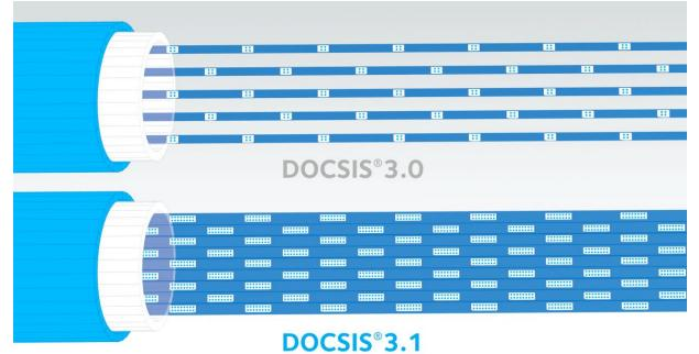
In addition to using enhanced signal processing techniques like 4096 QAM and OFDM, DOCSIS 3.1 allocates higher frequency spectrum for downstream and upstream data transfers. DOCSIS 3.0 used frequency band 5 MHz to 65 MHz for upstream and 85 MHz to 1002MHz for downstream, whereas DOCSIS 3.1 allocates 5 MHz to 204 MHz for upstream and 252 MHz to 1788MHz for downstream traffic.
