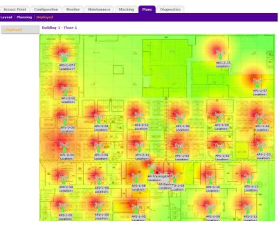
Figure 1: A "heat map" visualization of the signals from several Wireless Access Points.
