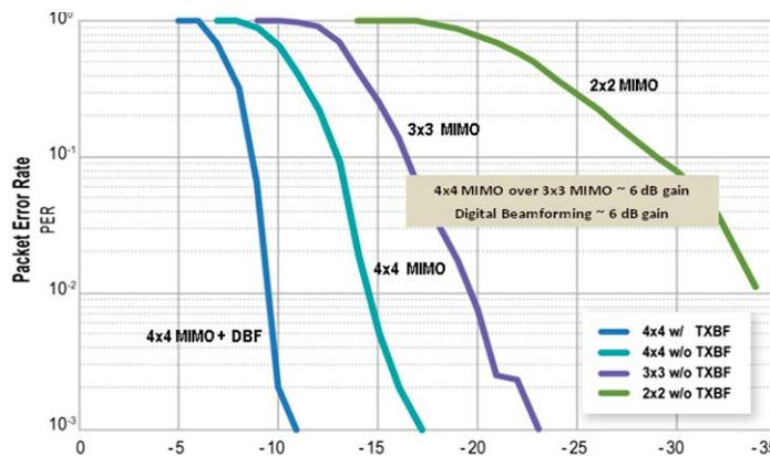
Figure 3. Packet Error Rate versus received SNR for various IEEE 802.11n systems (MCS12, 40 MHz, Channel D, 1000 Channels, 1000 byte packets)
